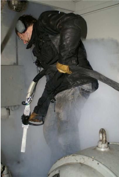
Abbildung 3 Abrasive blasting with dry ice pellets (09.08 Beck)
